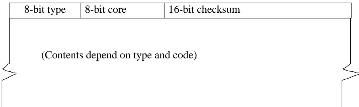
The 8-bit type code identifies the types of the message. This is followed by at least the first 28 byte of the packet that resulted in generation of the error message (i.e., the network –layer header and first 8 byte of the transport header). This payload is, for instance used by a sender that receives the ICMP message to perform Path MTU Discovery so that receives it may determine IP destination address of the packet that resulted in the error. Longer are also encouraged.
