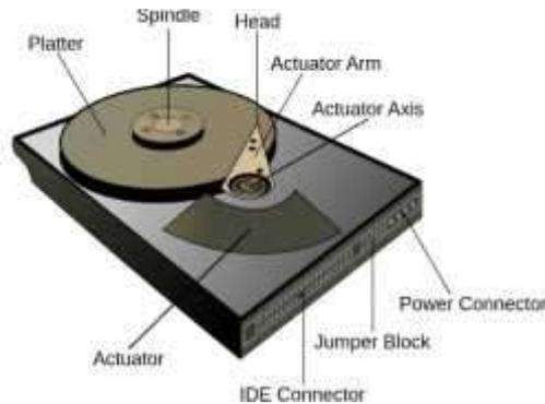
The platters are made from a non-magnetic material, usually aluminum alloy, glass, or ceramic, and are coated with a shallow layer of magnetic material typically 10–20 nm in depth, with an outer layer of carbon for protection. For reference, a standard piece of copy paper is 0.07–0.18 millimeters (70,000 –180,000 nm).
