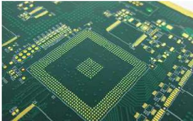
Components are generally soldered onto the PCB to both electrically connect and mechanically fasten them to it. The "card" is made of a material that does not conduct electricity, like fiberglass or plastic. Usually copper is etched inside the board between the layers of plastic, or on the surface of the board. This makes the electricity go only where it is wanted.
