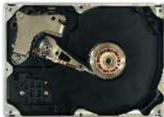
The actuator is a permanent magnet and moving coil motor that swings the heads to the desired position. A metal plate supports a squat neodymium-iron-boron (NIB) high-flux magnet. Beneath this plate is the moving coil, often referred to as the voice coil by analogy to the coil in loudspeakers, which is attached to the actuator hub, and beneath that is a second NIB magnet, mounted on the bottom plate of the motor (some drives have only one magnet).
